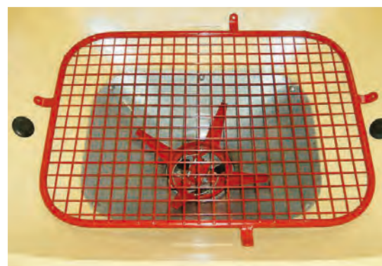
Agitator with safety grid
