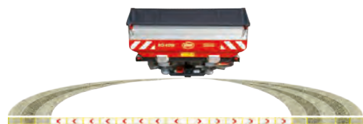
Switching off the sections outwards
