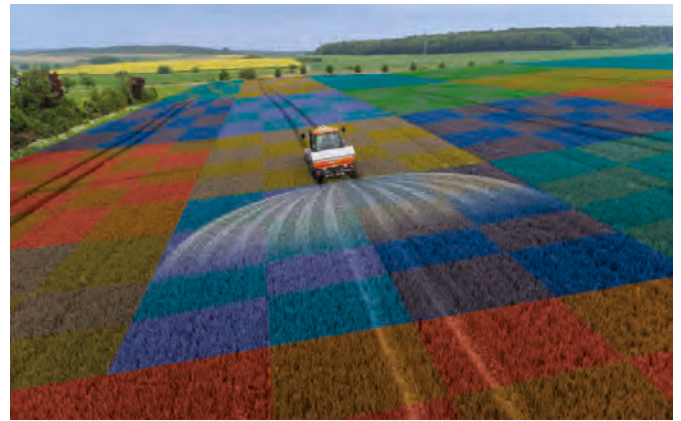
Variable rate control (MULTIRATE)
