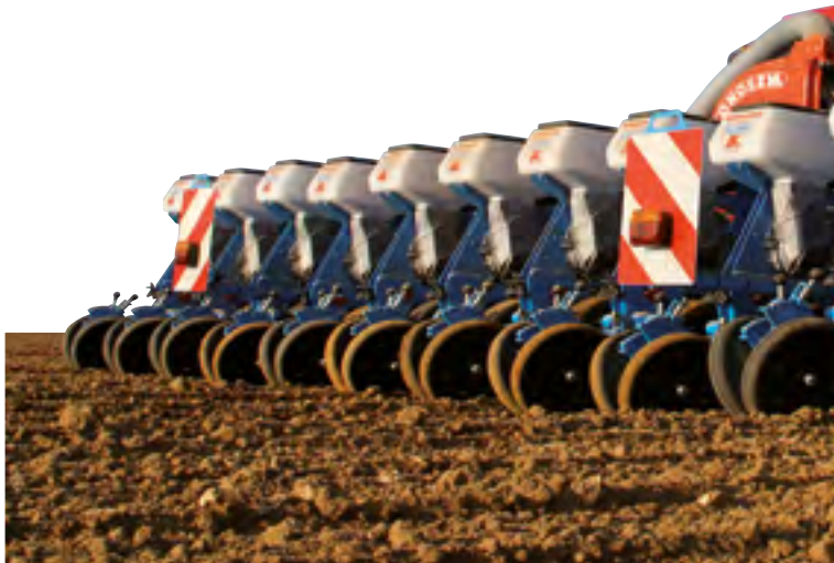
12-row Double bar folding planter (45 cm inter row spacing)
