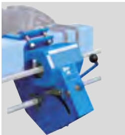
Central seed spacing gearbox Minimum inter-row spacings (1) : 33 cm
