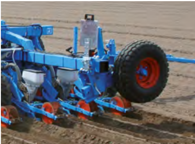
A lengthways transport carriage is available for wide-configuration planters. This transport carriage has a manual or hydraulic wheel lift.
