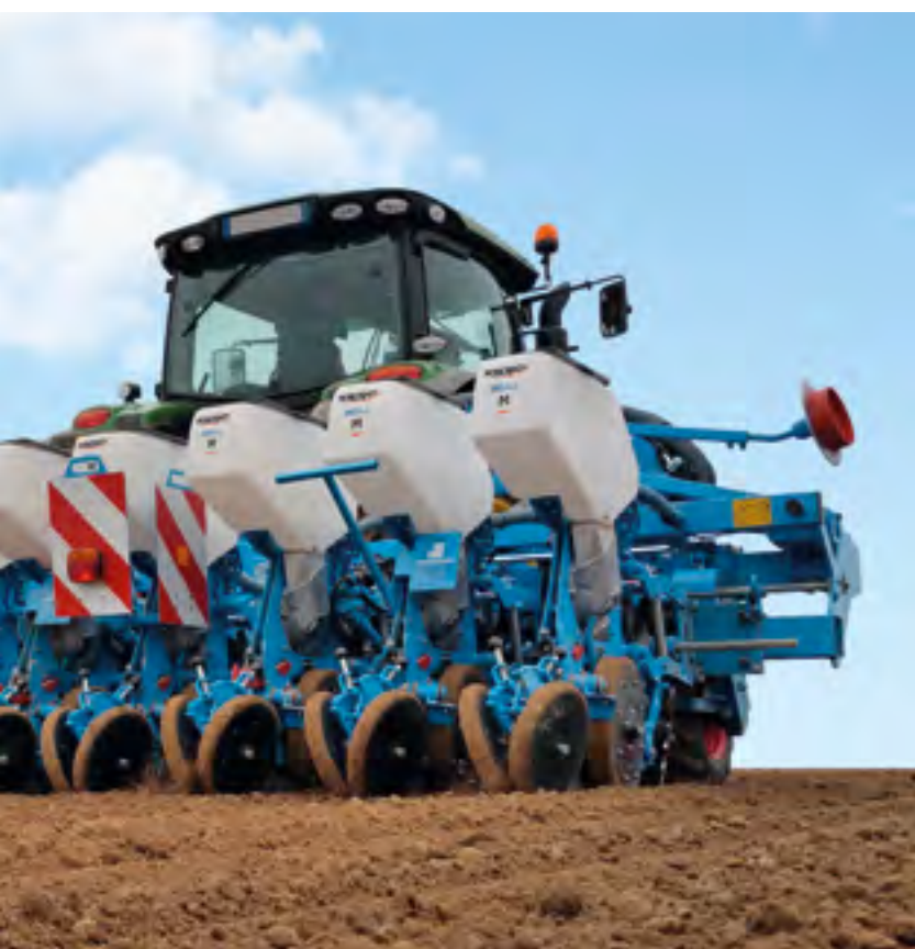
16-row TFC2 Comfort folding planter (37,5 cm inter row spacing) with equipment for DUO front-mounted fertilizer
