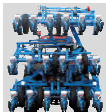
Three level folding MECA V4 18-row planter being transported
