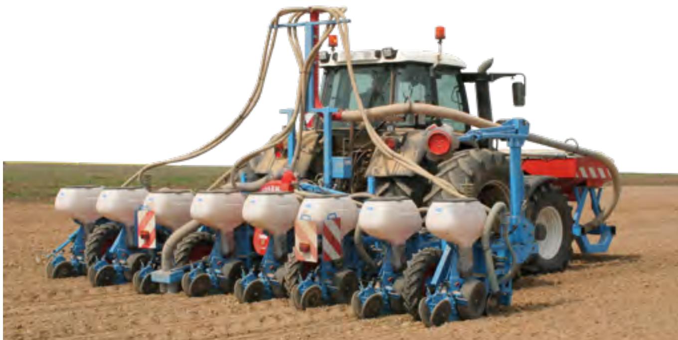
8-row folding planter with front fertilizer (inter row spacings of 75cm)
