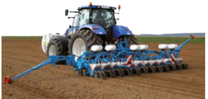
12-row double bar folding MECA V4 planter with Microsem
