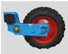
Adjustable wheel unit with 500 x 15 wheel Minimum inter-row spacings (1) : 36 cm Wheel clearance: 25 cm
