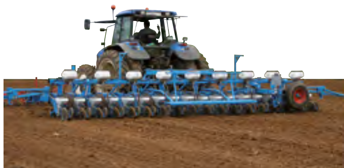
18-row rigid triple bar MECA V4 planter with Microsem and transport carriage
