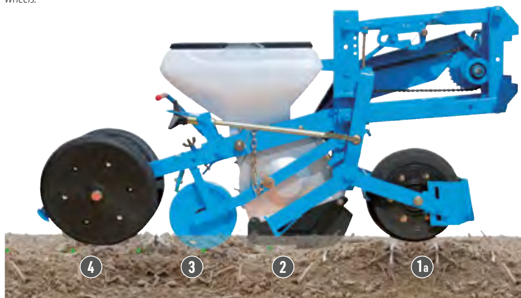
MECA V4 metering unit Front wheel 260x100 - Balancing System
