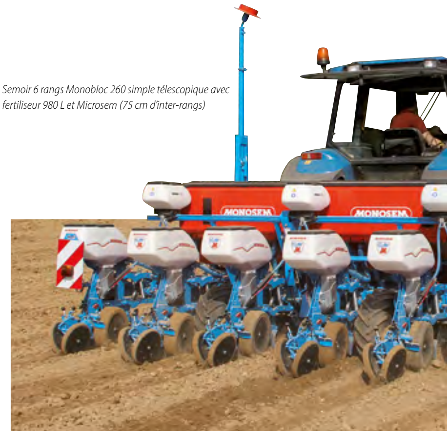
The Monoblock single telescopic frame The Monoblock single telescopic frame 260 has a 4,2m bar when working. When transported, the 1st and 6th rows retract for a transport width of 3,5m. This frame is also suitable for an uneven number of rows. The Monoblock 260 can be equipped with "High Capacity" fertilizer attachments.
