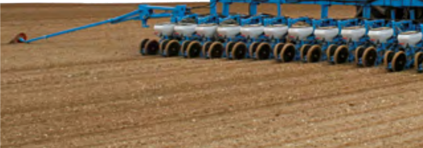
18-row rigid triple bar MECA V4 planter with transport carriage
