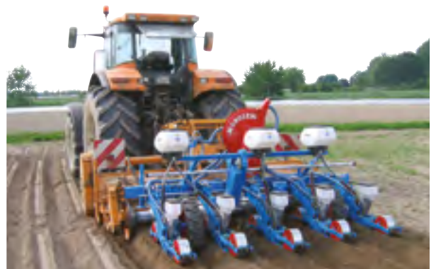
MS A Planter - Monobar rigid frame - 5 rows with Microsem
