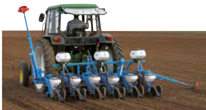
6-row rigid monobar MECA V4 planter with Microsem
