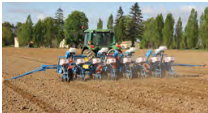
8-row Double bar folding planter (80 cm inter row spacing)
