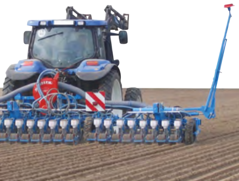
MS A Planter - Double bar folding frame - 3 x 8 rows
