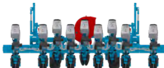
Example of configuration: 6 rows at 75 cm
