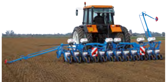
12-row compact folding MECA V4 planter with Microsem
