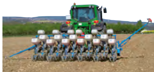
11-row rigid Monoblock planter (37,5 cm inter row spacings or 6 rows at 75 cm inter row spacing).
