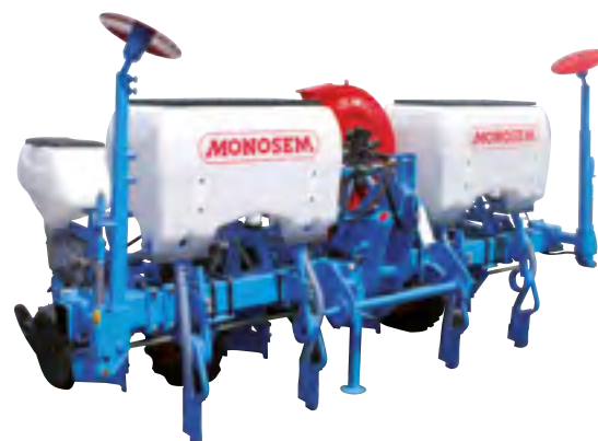
4-row rigid Monobar planter (75 cm inter row spacing)
