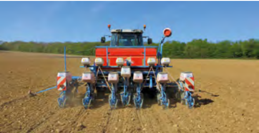
The mixed 6/7 row Monoblock2 version offers spacings of 75 or 80 cm in 6 rows and of 56,2 and 60 cm in 7 rows. Fertilizing is available for 6 and 7-row configurations.
