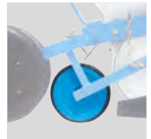
Rear cast iron concave unit with self-cleaning tyre
