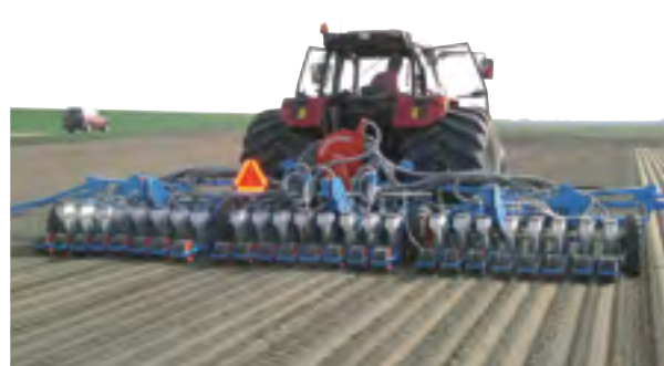
MS A Planter - Double bar folding frame - 3 x 8 rows
