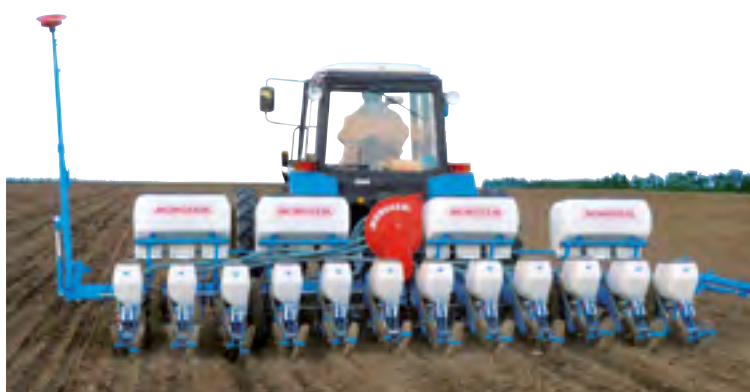
NC Technic Maize planter 12-row Monobar rigid frame (45 cm) - Fertilizer 4x175 L with knives
