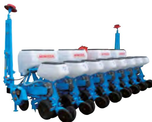
8-row rigid Double bar planter (70 cm inter row spacing)
