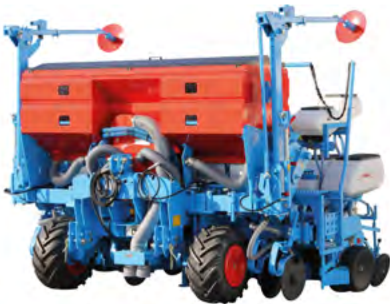
Planter with front wheel units for planting with reduced inter row spacings (up to 37,5 cm) or in stony soil conditions
