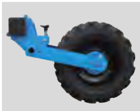
Adjustable wheel unit with 6,5 x 80 x 15 wheel Minimum inter-row spacings (1) : 45 cm Wheel clearance: 19 cm
