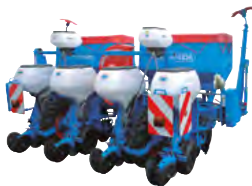
4-row planter with fertilizer (75cm inter row spacings)
