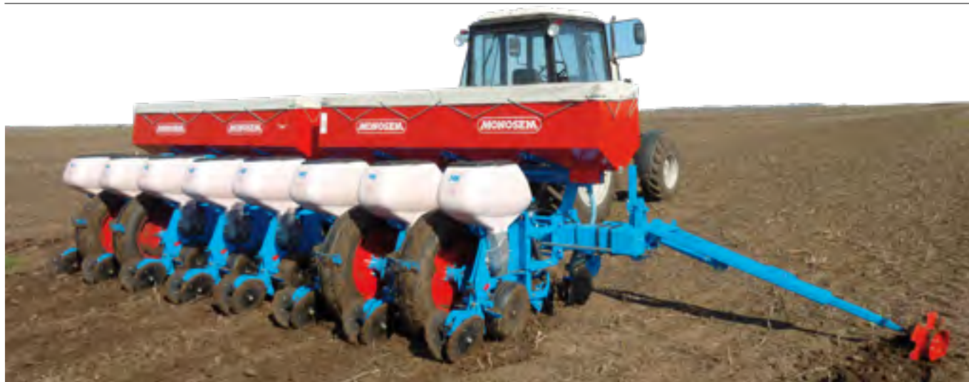
8-row pull-type planter with fertilizer (inter row spacings of 70cm)
