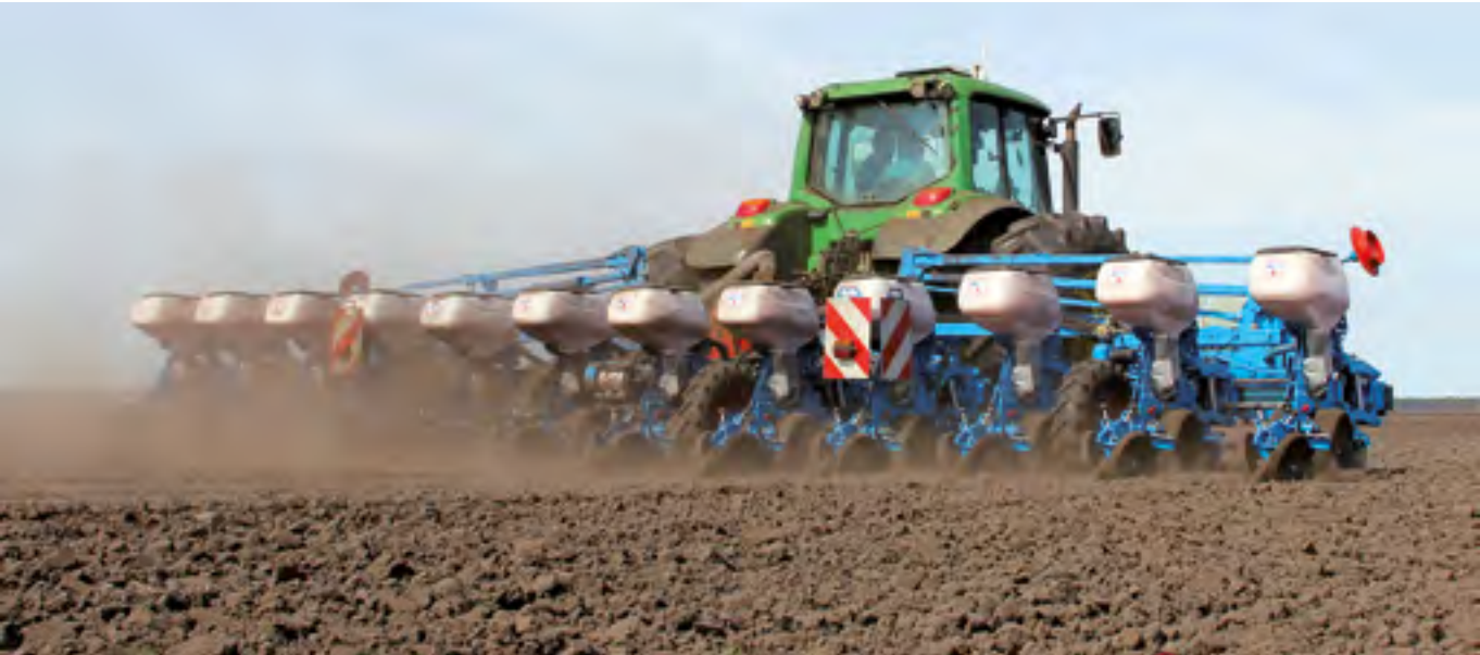
12-row CRT folding planter (80 cm inter row spacing)
