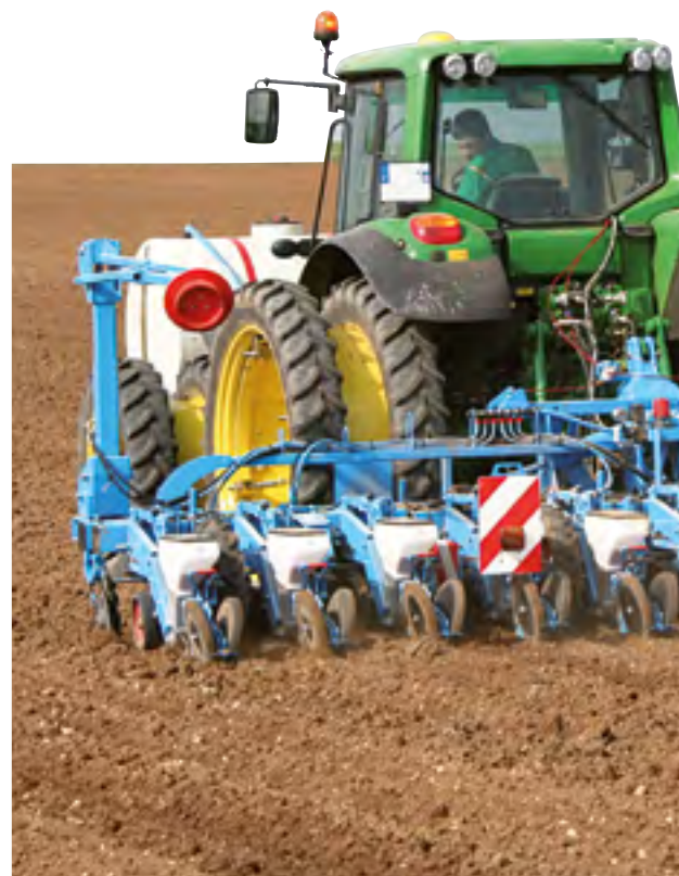
12-row double bar folding MECA V4 planter
