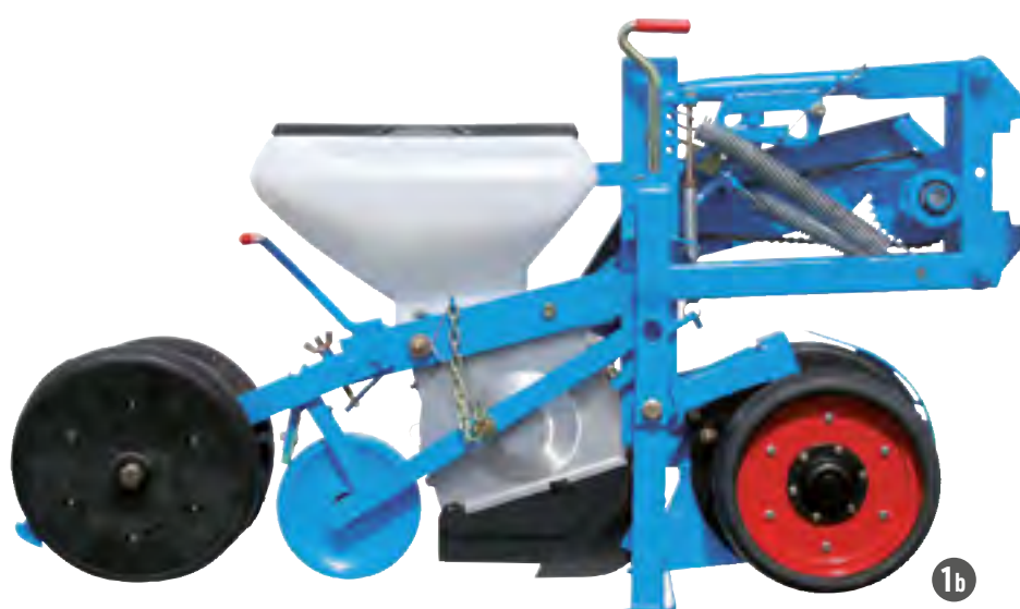
MECA V4 metering unit Front wheels 285x65 + double discs – Front depth control
