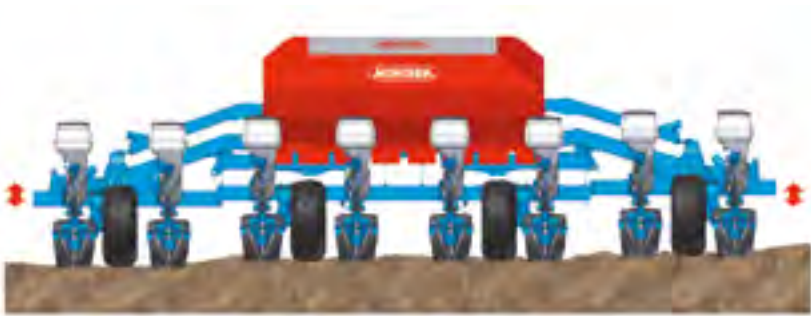
The floating Double bar folding and the floating TFC frames have independent wings with wheel units. This characteristic allows for a perfect following of the ground.
