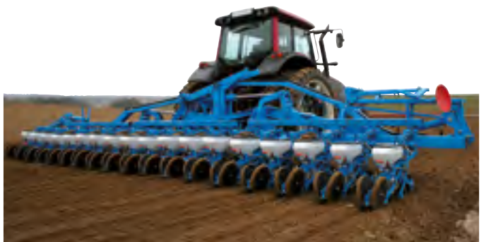
18-row three-level folding MECA V4 planter
