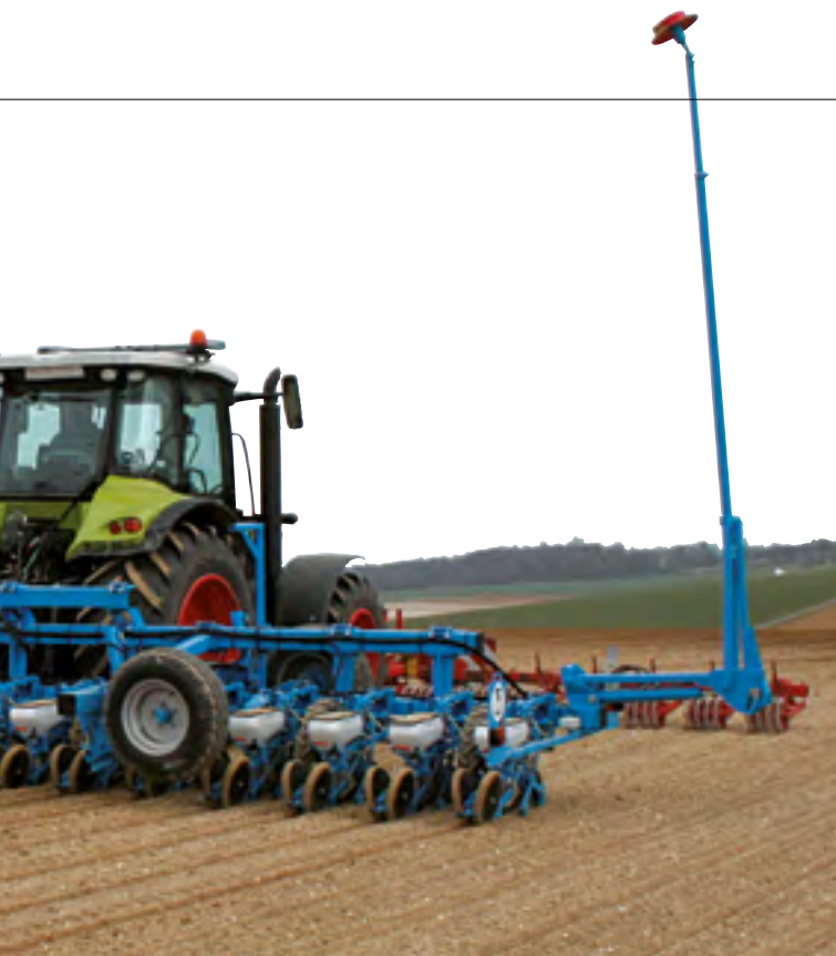
6-row rigid monobar MECA V4 planter with Microsem
