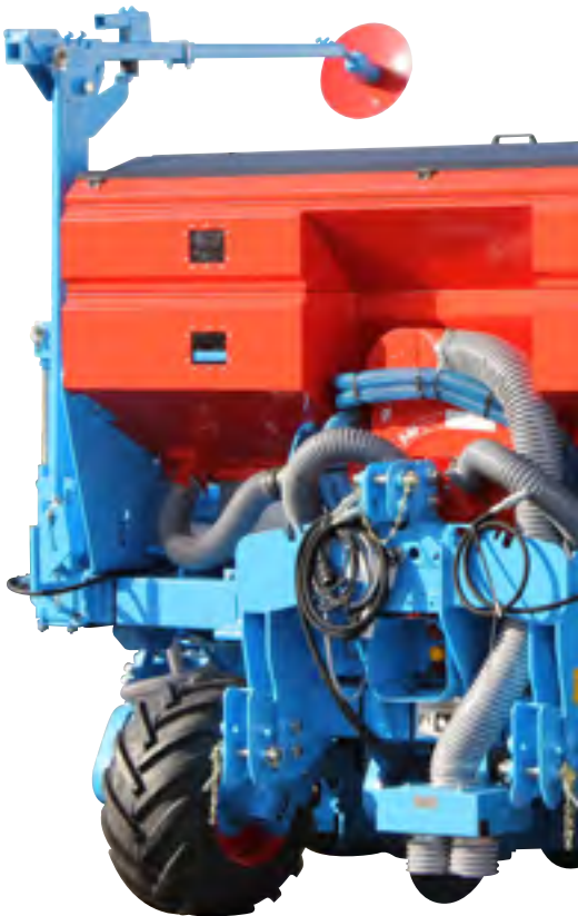
6-row Monoblock2 Comfort planter with fertilizer 1030L and Microsem handset (75cm inter-row spacings)
