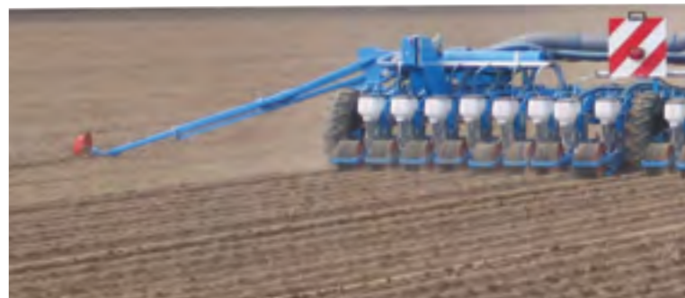
MS A Planter - Double bar folding frame - 3 x 8 rows
