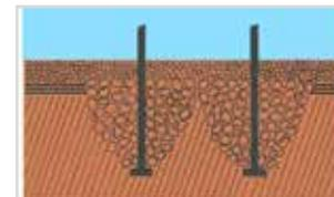
Deeper loosening relieves compaction by lifting and rearranging larger aggregates without bringing them to the surface. Narrower point, wing and angle options enable varying depth and aggressiveness.
