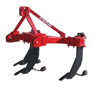
A kind of plough with no mouldboard, used to loosen the the soil at some depth below the surface without turning it over
